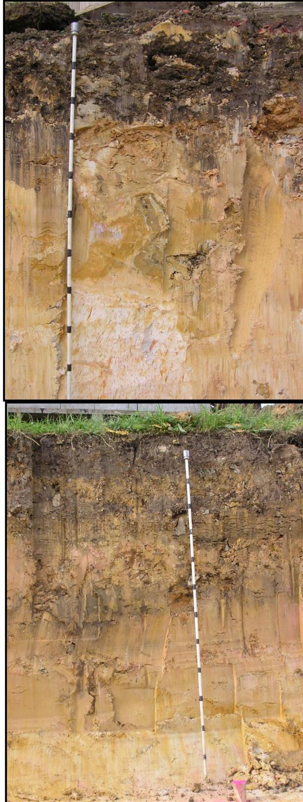
**Figure 7. Earthworking Ultic Soils in West Auckland (left) and Albany (right) has caused significantly reduced permeability to very low (Hydrological Class D); created massive soil structure; mixed topsoil with subsoil and regolith materials; and grey and red mottling has developed throughout the profile. (scale in 10 cm increments)**
