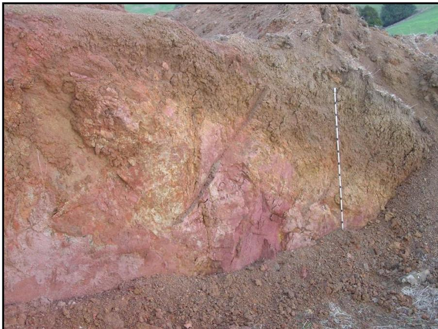
**Figure 2. A moderately permeable Granular Soil on red weathering in Waitemata Formation sandstone in the South Auckland area. (scale in 10 cm increments)**
