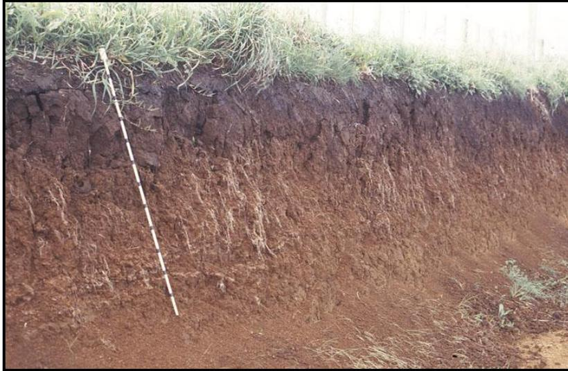
Figure 3. A moderately permeable, clayey Granular Soil, showing fine blocky structure and no mottling, from the South Auckland area. (scale in 10 cm increments)
